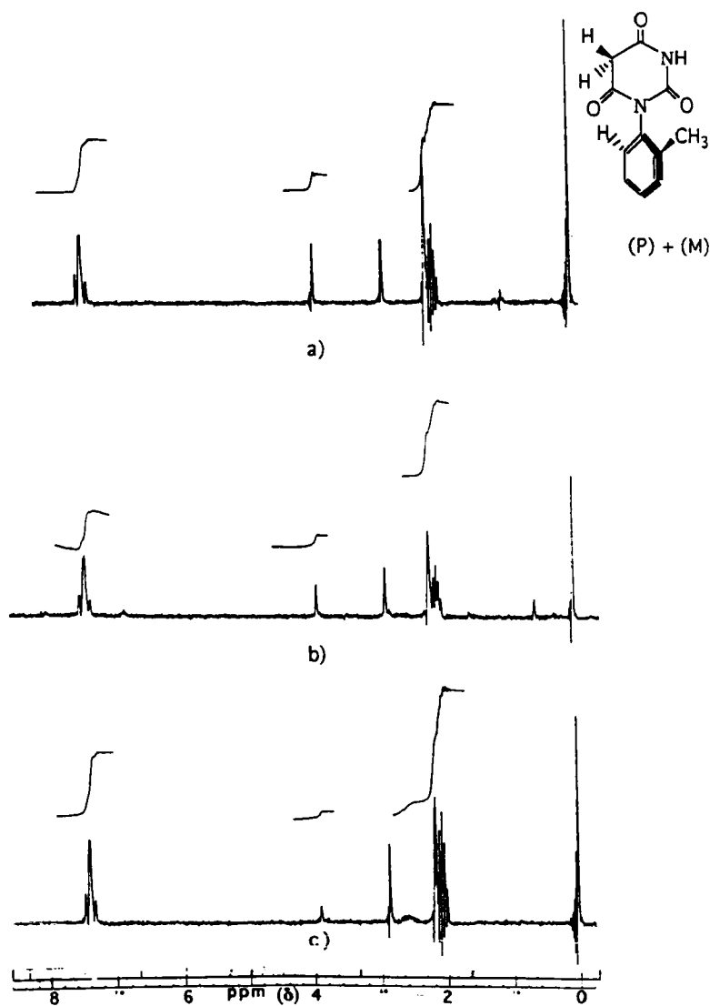
Fig.2. The 60 MHz 1 H NMR spectra of 1-( o -tolyl)barbituric acid in hexadeuteroacetone at 23°C taken after after a) 2 days, b) 4 days, c) 8 days.
